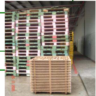
20 GPac pallet height vs 20 conventional wooden pallet height
